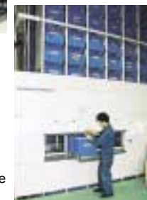
"Pick and Stocker" capable for storing 356 containers.
