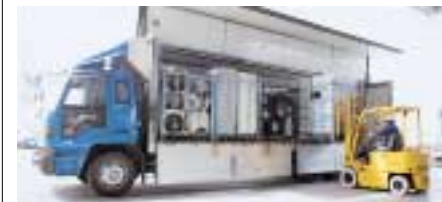
Six containers can be loaded on 10 ton truck.
