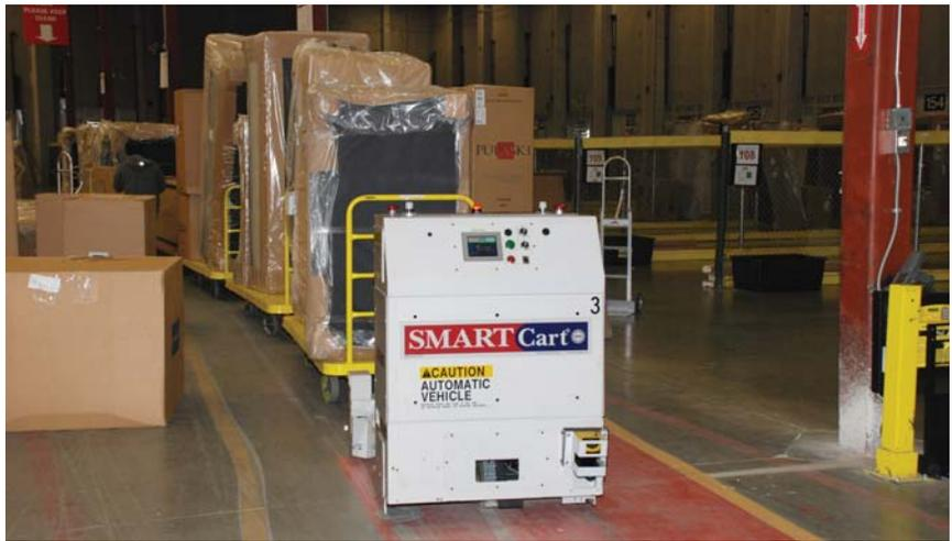
The SmartCarts are controlled by a computer system. A computer operator directs a SmartCart to one of six pick-up zones. After arriving at the assigned
