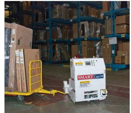
The furniture is manually unloaded at five drop zones. The associates have four minutes to unload the SmartCart or it starts beeping.
