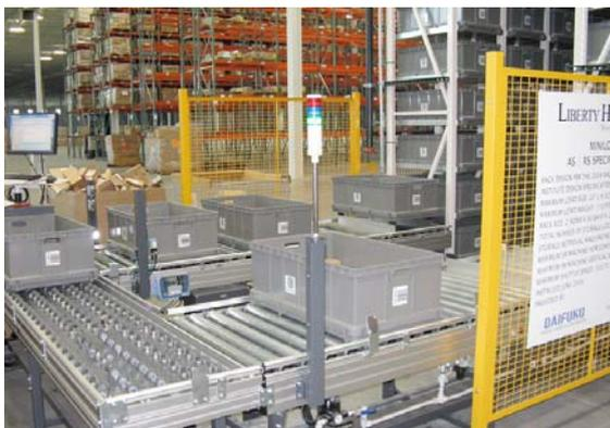
load Automated Storage & Retrieval System (AS/RS) would be sufficient to meet their current and future growth operation. The modified operation using AS/RS technology requires fewer personnel to pick orders than Liberty Hardware's previous manual operation, which consisted of multiple people manually picking from many aisles of conventional flow rack.
