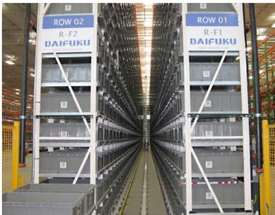
Not only does it control the operation of the crane, but it is the intelligent “brain” that directs picking efficiency. For example, the WCS retrieves SKUs that are part of single item orders before retrieving SKUs for multi item orders to ensure high throughput. The WCS interfaces with the Liberty’s own warehouse management system (WMS).
