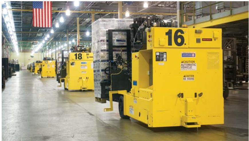
Building upon its intelligent AGV technology, Webb engineers designed the SmartLoader AGV to move loads into conventional trailers without guidance wires, lasers or magnets. The SmartLoader uses technology adapted from Webb's proven inertial guidance systems to reliably deliver palletized loads in multiple configurations into any standard over-the-road trailer.
