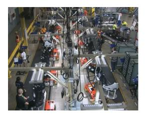
The advantage of being able to just pick up the magnetic tape and change the layout in a matter of minutes allows us to change an entire line over a weekend. When you look at the bang for the buck, you can't beat these SmartCarts.
