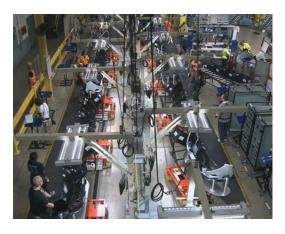
The advantage of being able to just pick up the magnetic tape and change the layout in a matter of minutes allows us to change an entire line over a weekend. When you look at the bang for the buck, you can't beat these SmartCarts.
