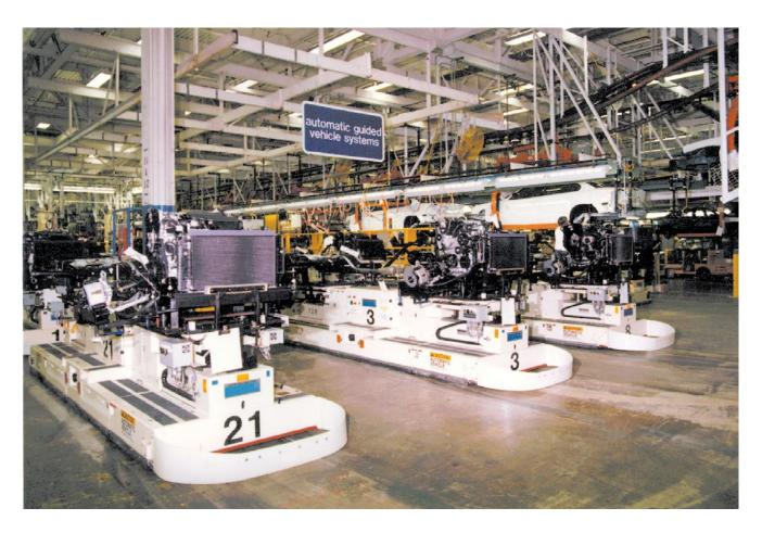
Daifuku's on-board assembly AGVs are the new standard for streamlining chassis assembly and chassis-to-body marriage operations. Current applications support complete sub-assembly build up as well as brake fill and test operations prior to chassis/body marriage. The system includes over 130 vehicles. A rugged design provides a flexible platform for guidepath system changes and model year changeover plans.
