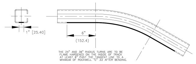
In addition, to ensure that the heat-treated area is not annealed, the track and yoke should not be welded in the heat-treated area as shown in Figure 2 below.
