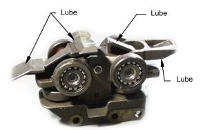
The following areas of the 6" Inverted Dog Magic<sup>®</sup> trolley require periodic lubrication:
