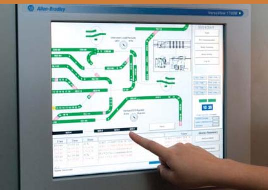
The WebbView® baggage handling control system integrates the four key elements of baggage system control: supervisory control, user interface, equipment control and manual encoding.
