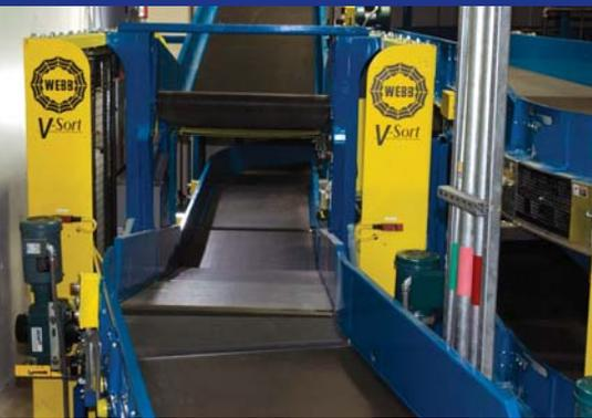
Vertical sort units are used in-line with the security scanning conveyor belts to remove suspect baggage to off-line baggage inspection.
