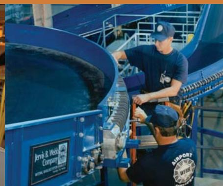
Webb Airport Services provides contract maintenance, spare parts and emergency repair services for baggage handling systems on a 24/7 basis.
