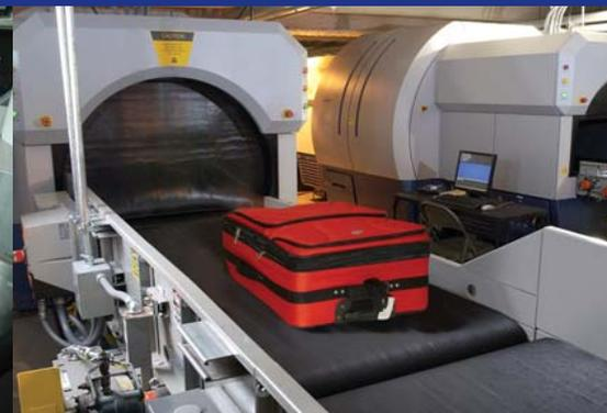
Every bag is fully screened through a multi-step scanning system that combines manual and electronic surveillance with x-ray and explosive detection equipment. Suspect bags are removed from the in-feed by high-speed Webb Vsort® vertical sorting conveyors.
