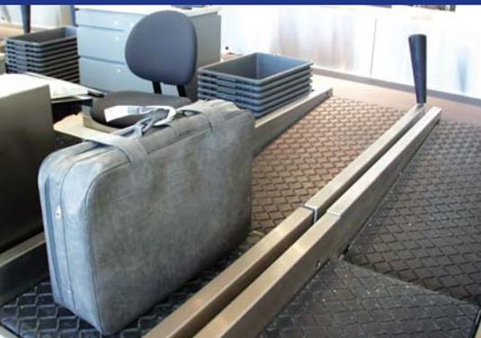
Our low profile, modular check-in conveyors consist of a scale conveyor, dispatch conveyor and a tipper to weigh, transport and lay down bags as they enter the gathering conveyor.
