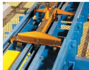
The three rail design stabilizes parts carriers.
