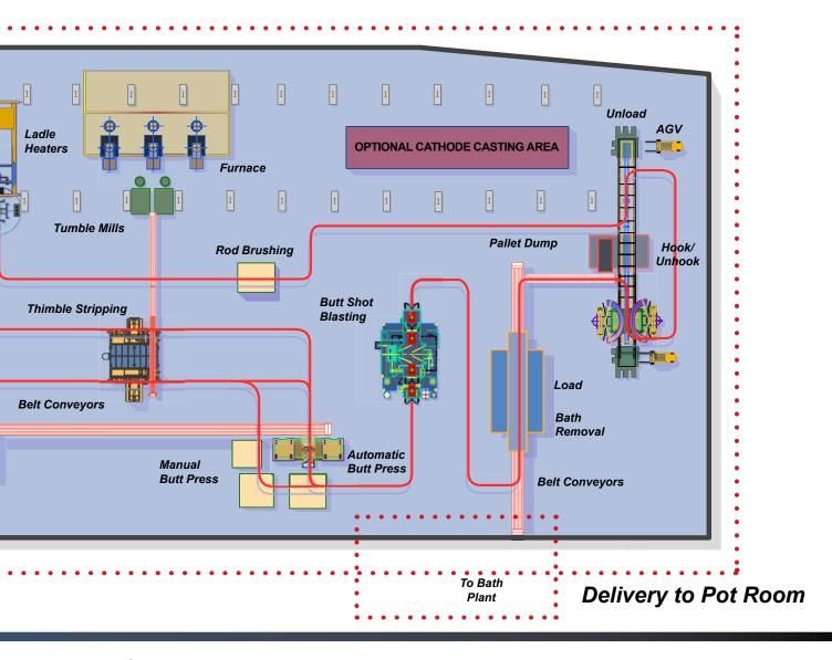
**Rodding Shop** – Daifuku manufactures and/or supplies process machinery for automatic load/unload stations, casting stations, shotblast units, stub heating, butt and thimble removal presses as well as rod repair operations. Power & free conveyors offer high volume throughput, extreme durability, and they're simple to operate and maintain.
