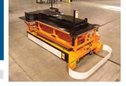
100 HD LHF Model: No. of AGCs: 28 + 8Operational: September 2010 System expansion April 2011 System Type: **Build Line for Batteries** Guide Path: Magnetic Tape System Active: Pending Load: Battery Cells and Completed Batteries Communication: Wireless 802.11a
