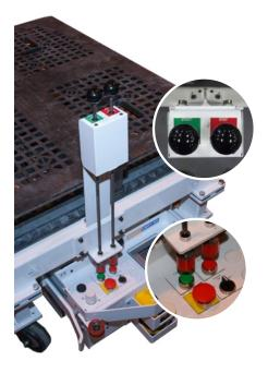
The mechanical pushrod assembly solves this problem by being permanently attached to the trailer giving the worker waist level access to the Start and Stop pushbuttons, when the trailer is attached to the AGC.
