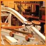
Track Switch – allows friction conveyor to operate like power & free
