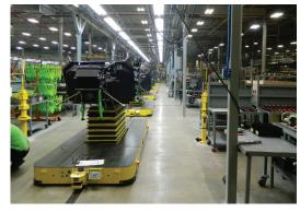
Patented "virtual bumpers" allow for a defined amount of space needed around the vehicle to ensure production is not hindered when vehicles stop for safety or work delays.
