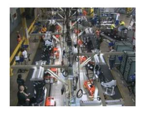
The advantage of being able to just pick up the magnetic tape and change the layout in a matter of minutes allows us to change an entire line over a weekend. When you look at the bang for the buck,
