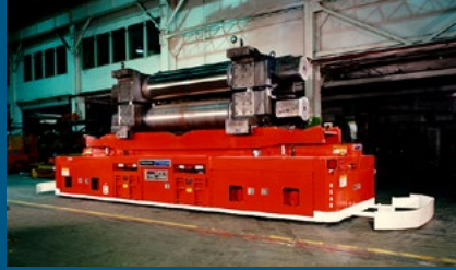
Work rolls are transported between Mill and Roll shop with less chance of damage. Backup rolls can be transported in the same manner.
