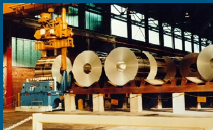
Utilizing an automated crane for direct loading of coils, this vehicle transports single coils between multiple processing centers. Load capacity of the vehicle shown is 60,000 pounds.
