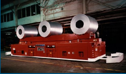
Various size coils at the finishing end of a mill are handled with this versatile coil handling AGV. The same vehicle is capable of handling work rolls.
