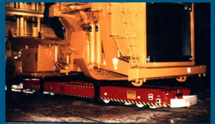
This ultra low profile vehicle moves 95,000 pound earth grader and dump truck chassis between various assembly operations.
