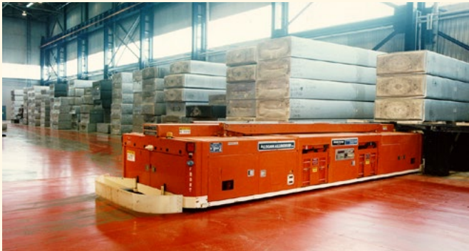
Aluminum ingots are delivered to a storage area and automatically unloaded by a vehicle mounted lift/lower deck.
