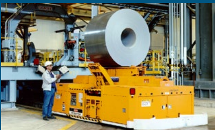
Steel coils weighing up to 120,000 pounds move between load stands serviced by automatic cranes and automated process equipment.
