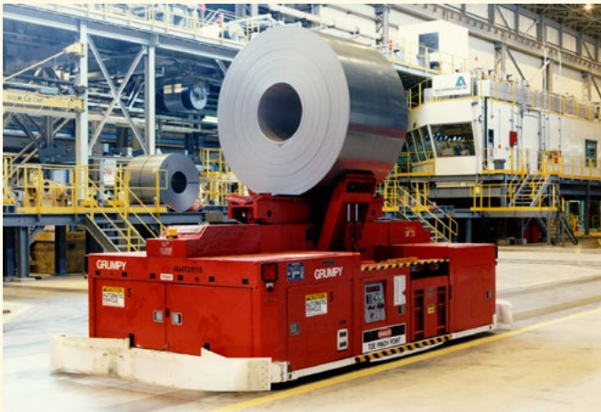
These AGVs interface with cantilevered pick/drop stations that can be supplied as part of the AGV system. A 100,000 pound load capacity AGV is shown transporting a steel coil.
