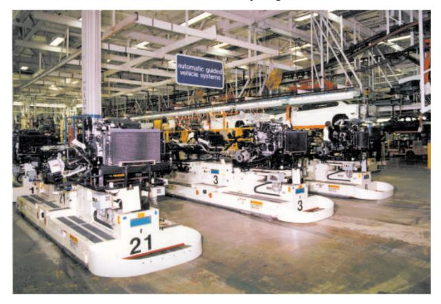
Jervis B. Webb Company's on-board assembly AGVs are the new standard for streamlining chassis assembly and chassis-to-body marriage operations. Current applications support complete sub-assembly build up as well as brake fill and test operations prior to chassis/body marriage. There are over 130 vehicles currently in operation and more are slated to go on-line in the future. A rugged design provides a flexible platform for guidepath system changes and model year changeover plans.
