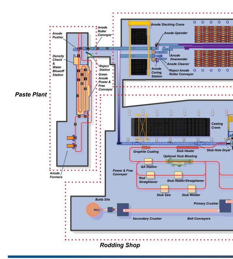
**Paste Plant** – Power & free conveyors transport green anodes from vibrocompactors through the cooling tunnel and to the roller conveyor. Only the anode itself is exposed to the cooling fluid bath. The operating components of the overhead conveyor system are located away from the coolant water to help extend conveyor life and increase operating efficiency.
