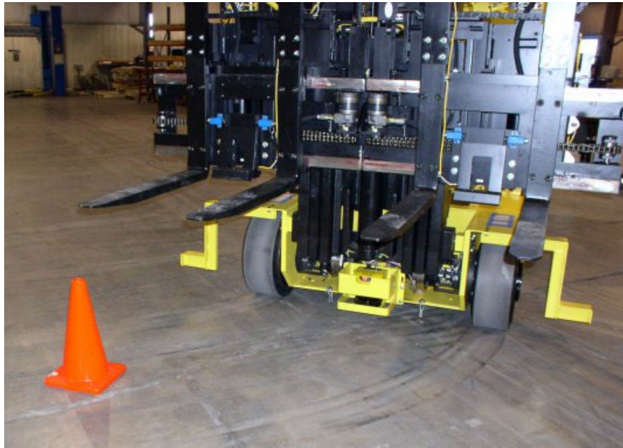
Figure 4: Illustrating proper traffic cone placement
