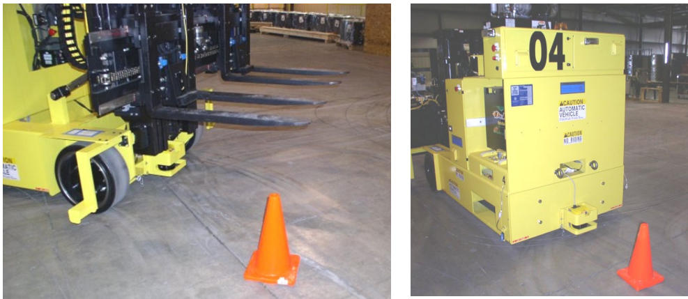
Figure 1: Illustrating proper traffic cone placement.
