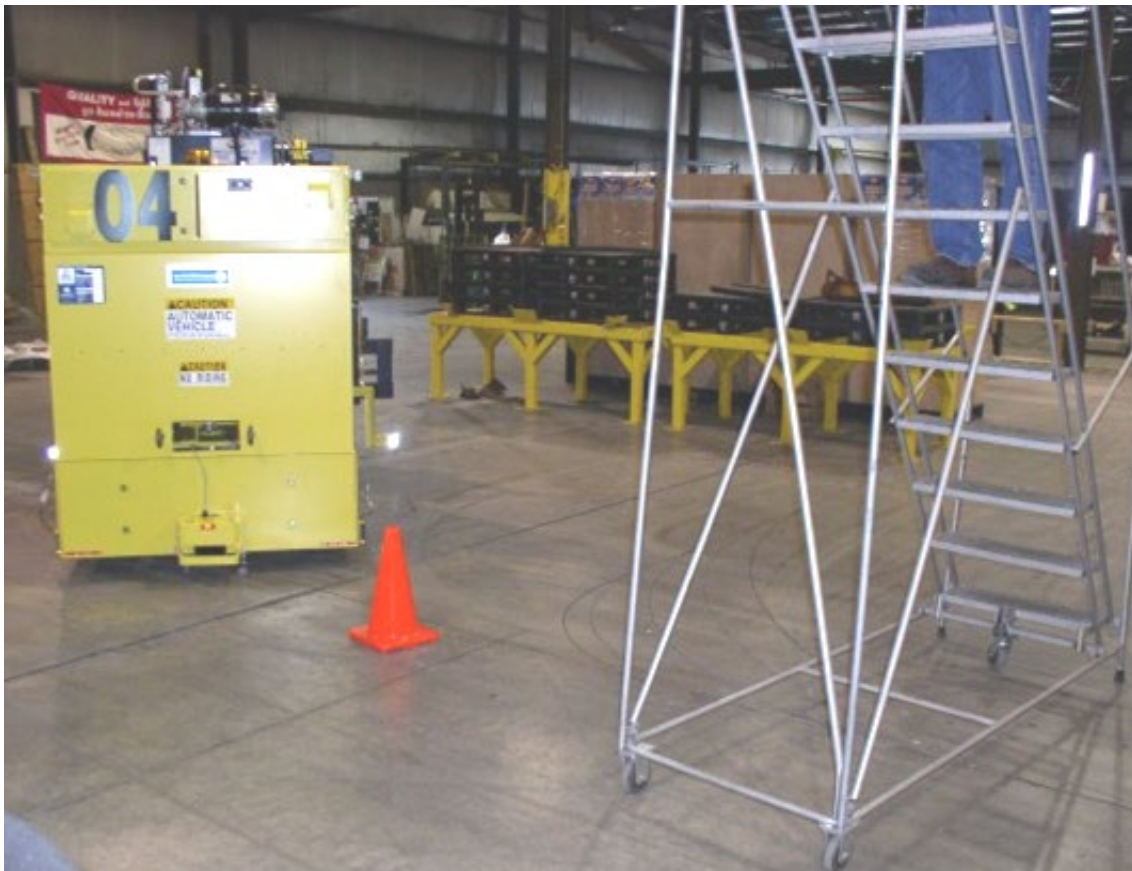
Figure 3: Illustrating proper traffic cone placement.
