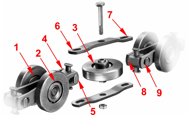
Figure 1" Lubrication Points for Unibilt® Chain
