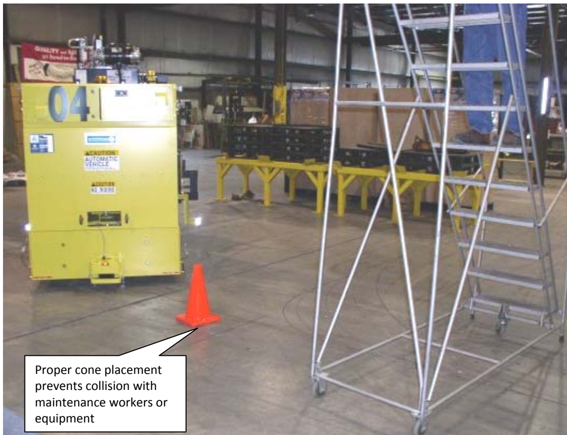
Figure 3: Illustrating proper traffic cone placement.
