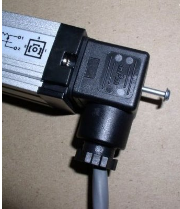
Figure 7: Secured Using Screw
