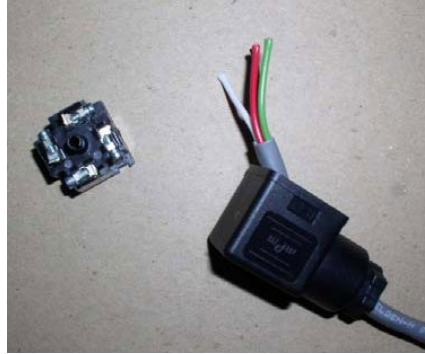
Figure 2: Cable Pushed Through
