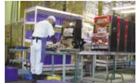
'Goodshelf' installed in dismantling plant: Shelves are tilted to keep the better view of contents in 'FS Container'
