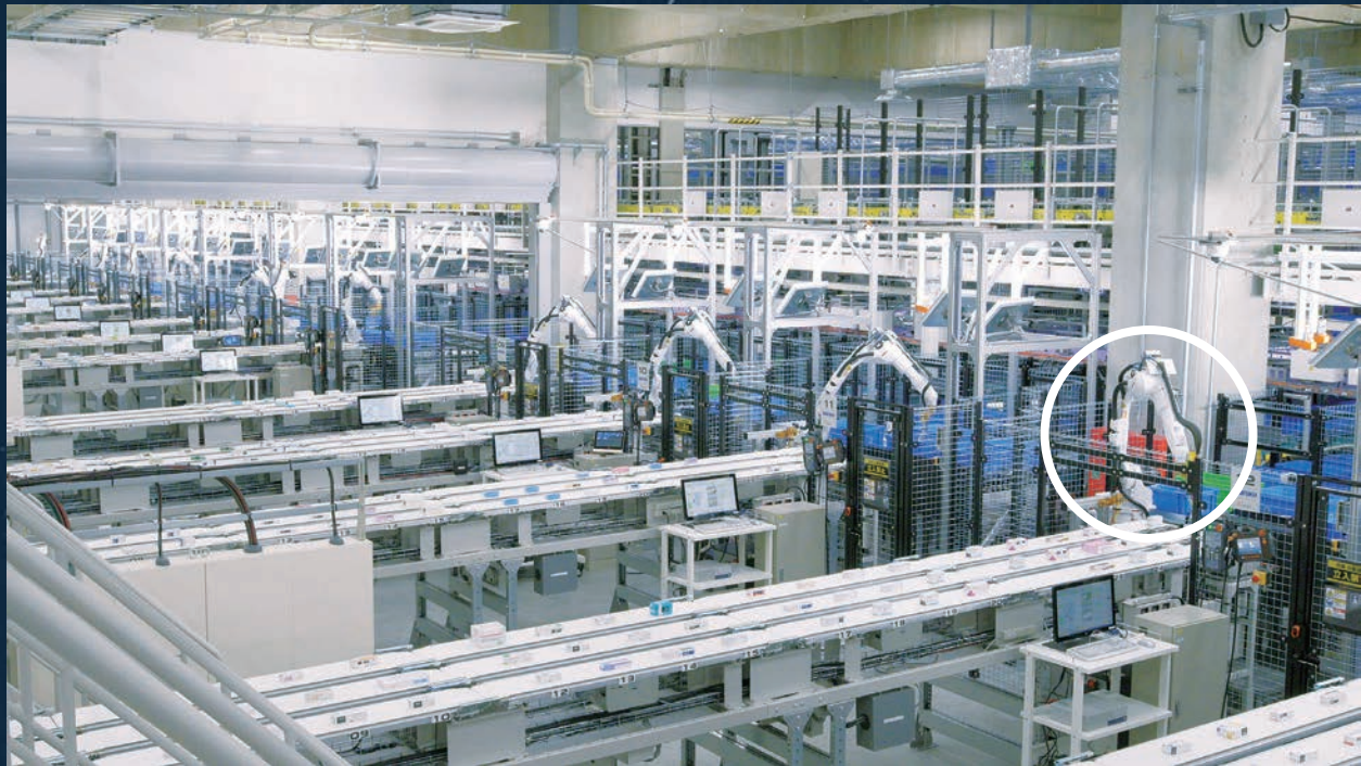
Robots pick individual boxes and deposit them on the conveyor, after which they are consolidated into customer orders.
