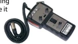
**SmartSteer** – CartTools directing the AGV to intentionally leave the magnetic tape path. It allows maneuvers like pivot turns and ignoring floor problems when in full automatic operation.
