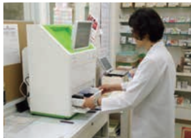
(Picture 1) Automatic checking system for dispensaries – audit
