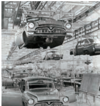
Chain conveyor system delivered to Japan's first passenger automobile factory
