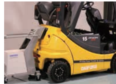
(Picture 2) Wireless battery charging system for electric forklifts – D-PAD
