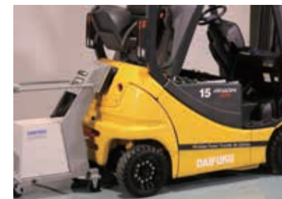
(Picture 2) Wireless battery charging system for electric forklifts – D-PAD
