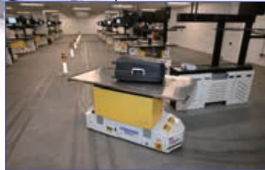
AGV-based mobile inspection table
