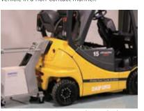
(Picture 2) Wireless battery charging system for electric forklifts - D-PAD
