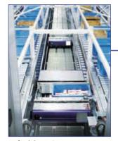
**As/RS\* for picking operations**Provides products in a timely manner to piece-picking robots.
