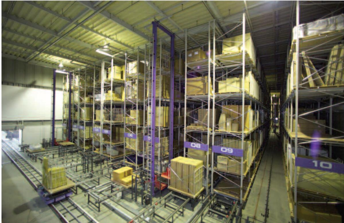
Automated Storage/Retrieval Systems (AR/RSs), core equipment for streamlining distribution. These systems are being actively used in Japan and throughout the world in various product manufacturing and distribution processes, including in the IT, food, beverage and pharmaceutical industries.
