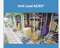
Daifuku's Unit Load AS/RS automatically transports products and parts in high-rise racks. By effectively using the height direction, it is possible to improve storage efficiency.
