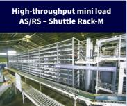
Daifuku's Shuttle Rack-M is a fast, vehicle-type AS/RS designed to provide temporary storage, sorting, and sequencing functions. Unlike the conventional stacker crane type AS/RS, its shuttle vehicles with a transfer function, which are arranged on a rack, transport in the depth direction and put it in and out of the shelves. It can be used for various load profiles, such as cardboard cases and trays.
