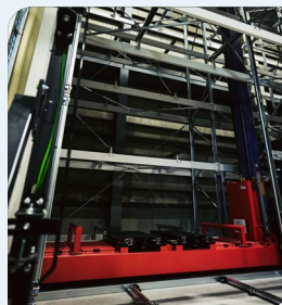
Automated warehouse capable of handling long items
