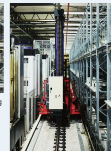
The inter-process transfer of supplying materials from the automated warehouse to processing machines and the storage of processed parts back in the automated warehouse have been automated.
