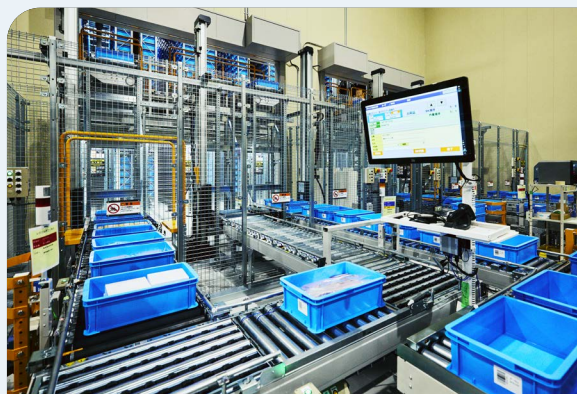
Parts centers store and sort around 38,000 different components.
