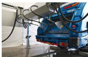
Shower Hopper cleaning the inlet
