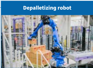
Picks cardboard boxes from a pallet retrieved from an AS/RS
