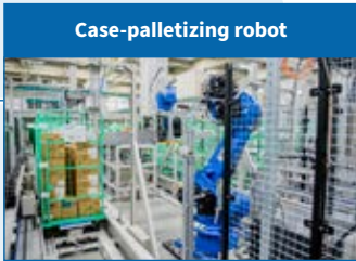
Rapidly palletizes cases of various shapes and sizes
