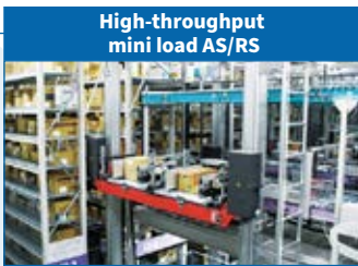
Stores various-sized cardboard boxes and facilitates case shipping
