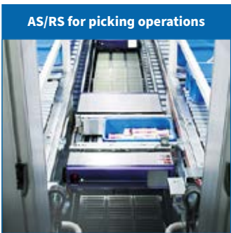
Provides products in a timely manner to piece-picking robots
