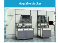
Storage for containers (magazines) for supplying and storing bonding\* materials
