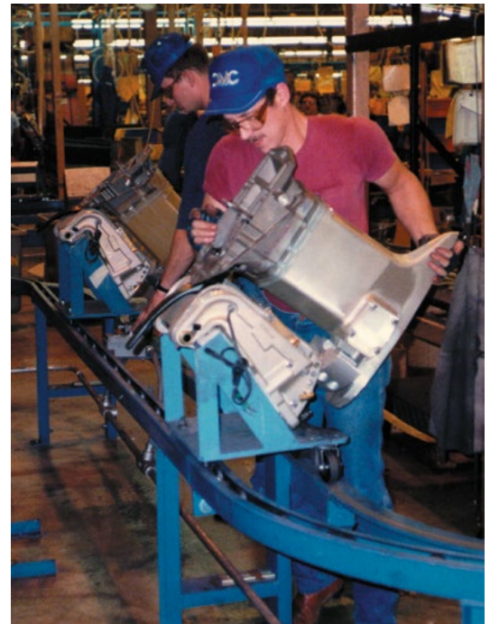
A two-rail floor mounted, tow style inverted continuous flow conveyor system, guides out-board motor units through assembly.
