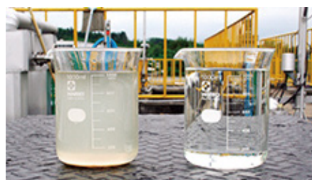
Effluent before (left) and after (right) treatment
