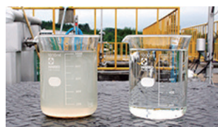
Effluent before (left) and after (right) treatment
