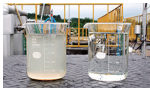
Effluent before (left) and after (right) treatment
