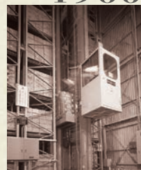
The Rackbuil installed in a Matsushita Electric Industrial facility
