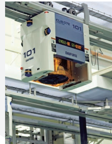
Cleanroom transport systems for semiconductor production
