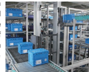
Mini load AS/RS for temporary storage of shipping containers
