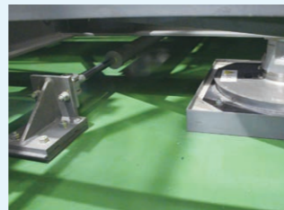
Parts composed of oil dampers and ball bearings
