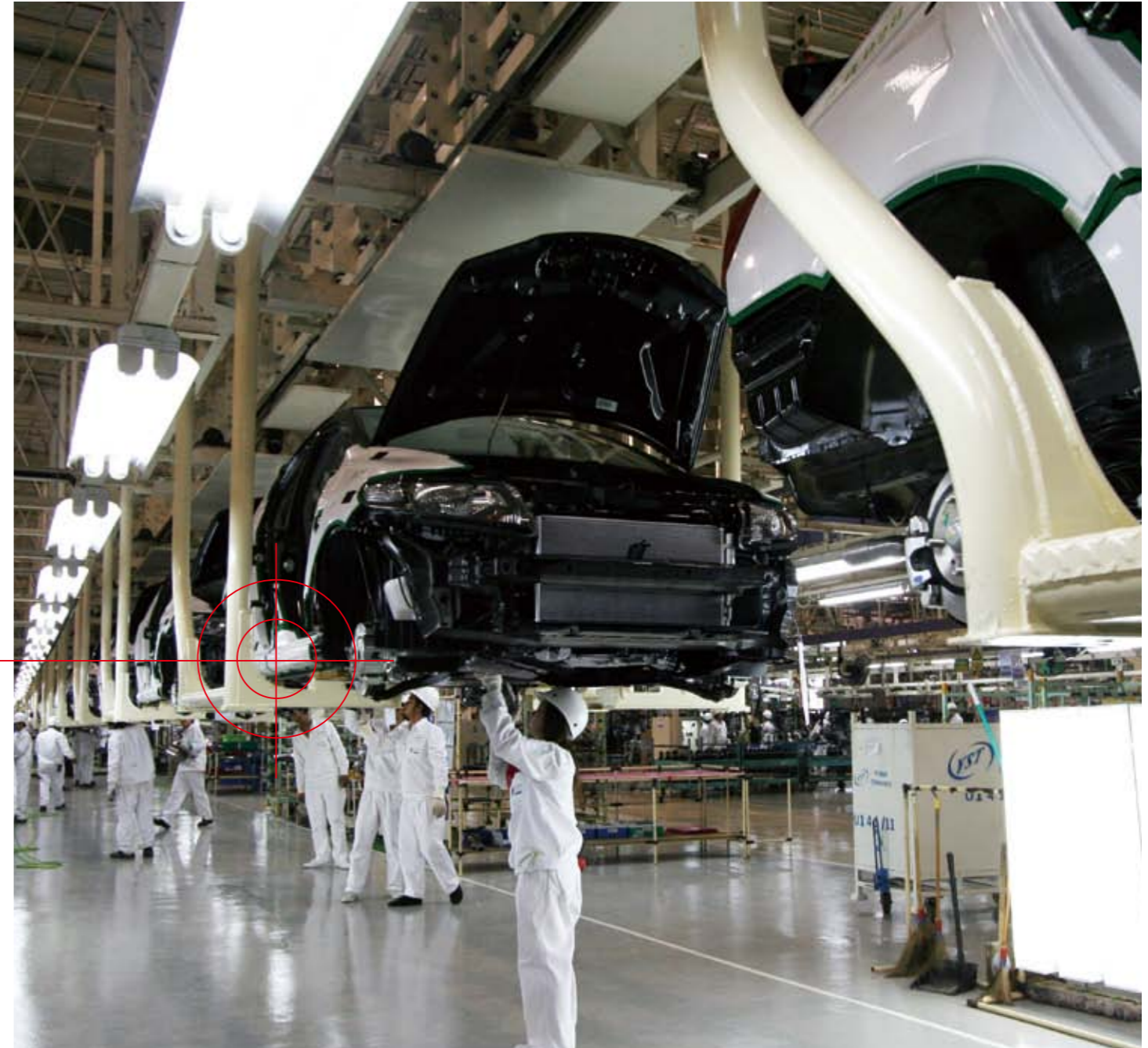
Daifuku's power & free chain conveyor system on the chassis line for engine and underbody assembly (450 m in conveyor length, with 55 carriers)
