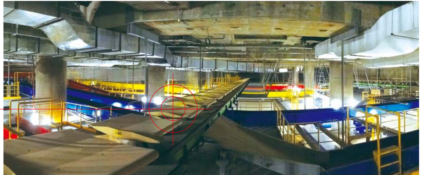
Two Tilt Tray Sorters totaling 580 meters and 532 trays
