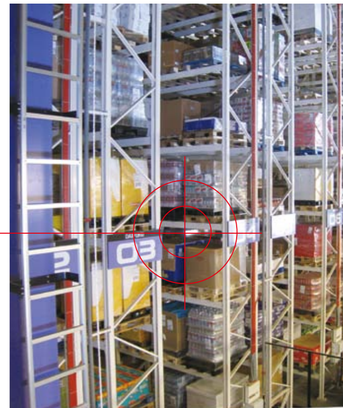
Unit load AS/RS with 13 stacker cranes and 26,000 pallet capacity
