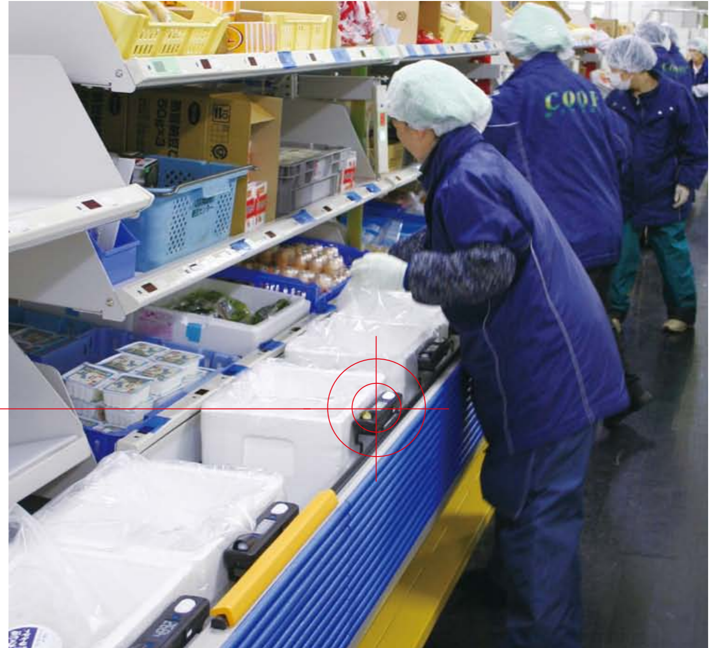
Refrigerated line incorporating the eye-navi . Displays on collection boxes and shelves are synchronized.
