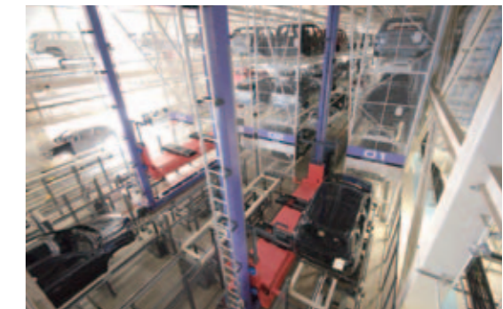
Unit load AS/RS with 108-vehicle storage capacity retrieving specified vehicle bodies to transport them to assembly lines in about one minute
