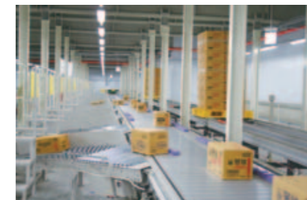
Surfing Sorter handling cases retrieved from the AS/RS by shipping destination
