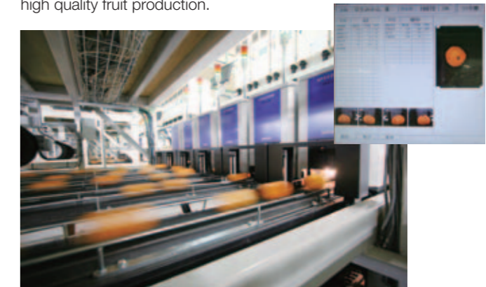
External quality sensors photograph and instantly analyze fruit to determine shape, color, damage and size.
