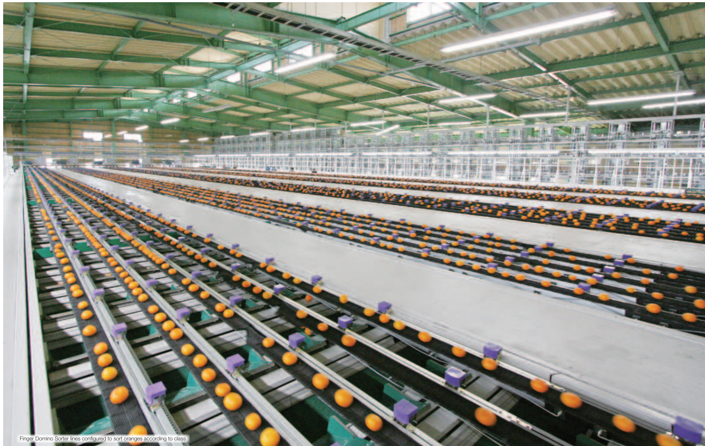
External quality sensors photograph and instantly analyze fruit to determine shape, color, damage and size.
