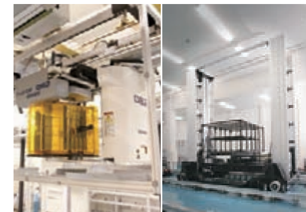
Clearway and Clean Stocker for semiconductor and FPD production lines using HID
