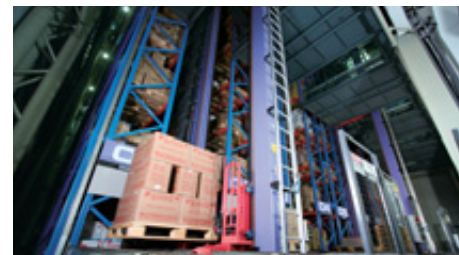
Unit load AS/RSs form the core of the center's storage and replenishment functions.
