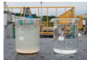
Effluent before (left) and after treatment
