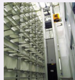
Storage system for semiconductor manufacturing fabs—Clean Stocker
