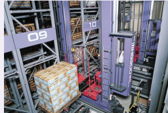
Rack-supported building AS/RS—Rackbul System
