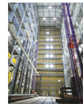
An S/R machine running at Daifuku's high-rise research building at the Shiga Works
