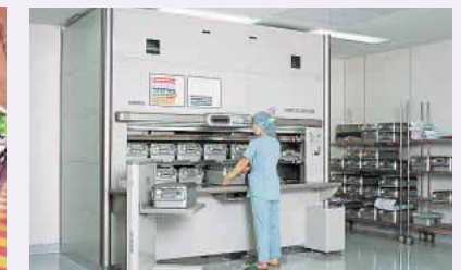
Vertical rotary rack for surgical instruments storage—Vertical Carousel
