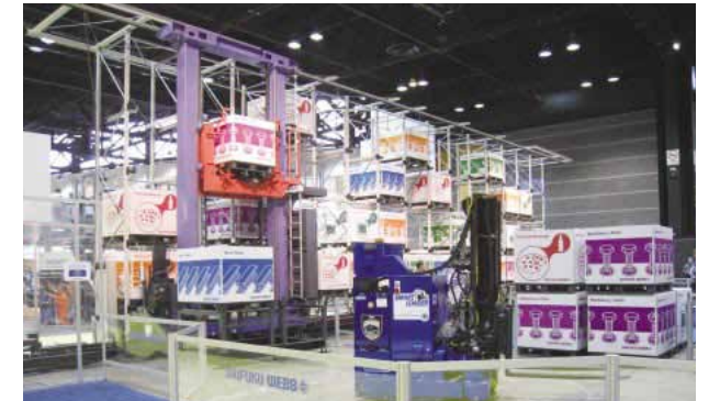
At ProMat, Jervis B. Webb's SmartLoader handled loads in sync with the operation of Daifuku's unit load AS/RS.
