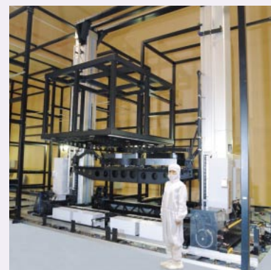
Storage system for FPD manufacturing fabs—Clean Stocker
