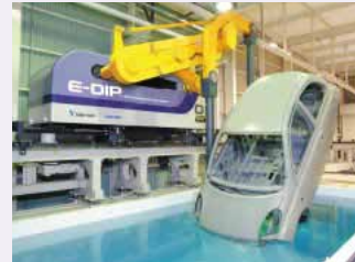
Environment-friendly paint system—E-DIP
