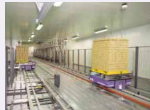
High-speed rail—guided vehicle—Sorting Transfer Vehicle
