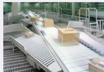
High-speed sorter—Jet Surfing Sorter
