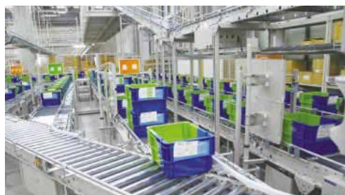
A conveyor line of cases sorted for designated stores
