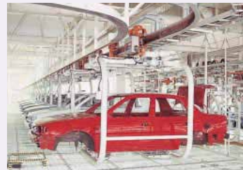
Electrified monorail system—Ramrun
