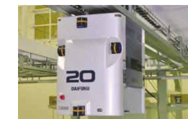
Transport system for semiconductor manufacturing fabs—Cleanway
