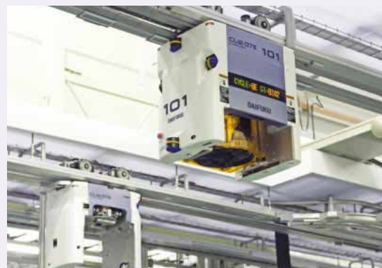
Transport system for semiconductor manufacturing fabs—Cleanway
