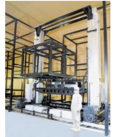
Clean Stocker for LCD manufactures
