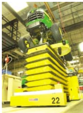
SmartCart automatic guided vehicle (AGV) for assembly plant use
