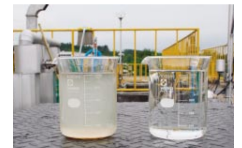
Before (left) and after (right) drainage treatment
