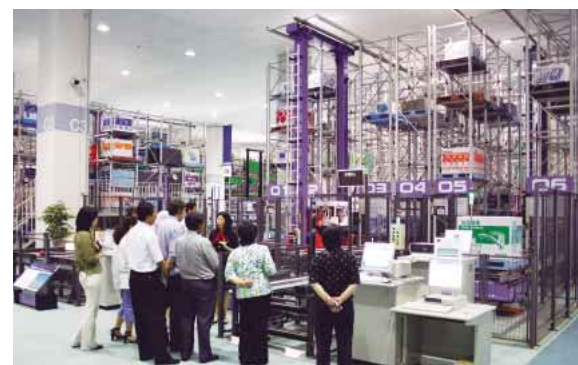
Unit load AS/RS, pallet-type automated warehouse
