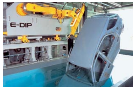
E-DIP enables better control when immersing and removing the body of the automobile from the tank
